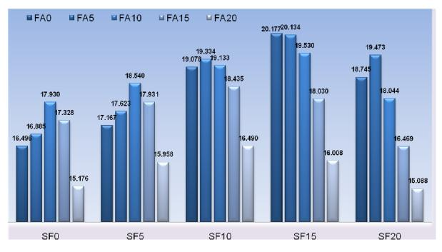
Figure 3. Change in compressive strength of 0-5-10-15 and 20% silica fume substituted series with increasing fly ash.
